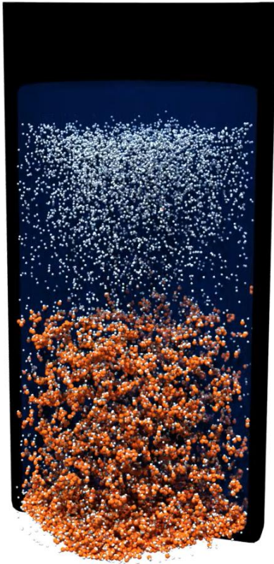
Slurry Settling in a Storage Tank
