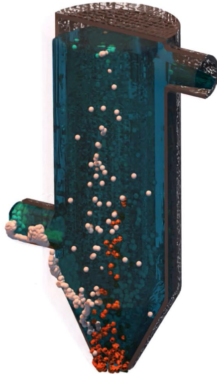
Particle classification by Elutriation
